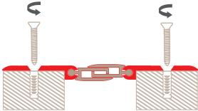
The fastening screws recommended have been dimensioned according to the efforts that the joint will have to support during its utile life. It you choose to use alternative fastening screws , please take this into account.
