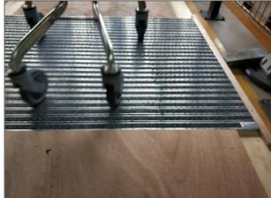
This test is carried out by moving a shopping cart loaded with 80 kg on a technical mat Novomat® 15 textile finish in a three meter long round trip. After 100,000 cycles it is confirmed that there is no structural damage to the aluminum and that the carpet has normal wear and tear for use.
