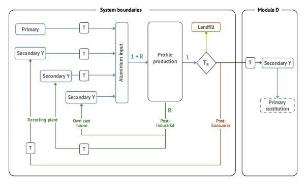
R - Process losses T<sub>R</sub> - Recovery Rate Y - Smelting yield T - Transport
